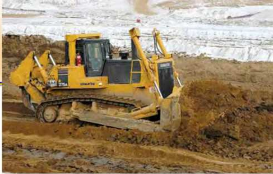
Komatsu dozers are a staple in the M.A.P. companies' fleets. This D375A-5 removes overburden at Inland Cement in Edmonton. "The D375 and D155 are excellent for stripping and moving mass amounts of dirt quickly," said Equipment Manager Paul Matera.
